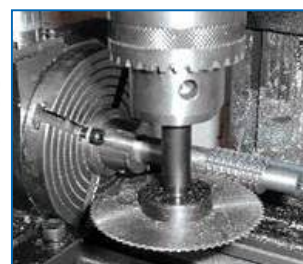
Saw holder being vertically mounted on a milling machine
